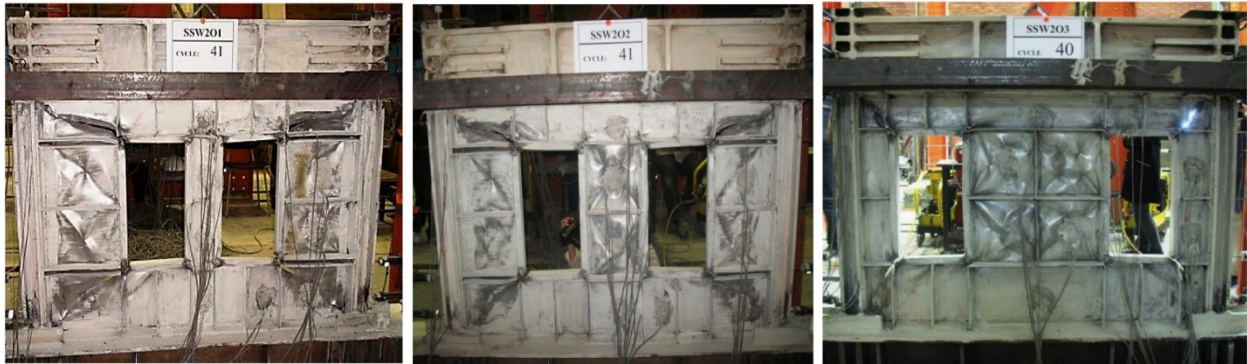
Fig 2.18. Deformed shapes of SSW2O1 (left), SSW2O2 (middle) and SSW2O3 (right) during the tests (Sabouri-Ghomi and Mamazizi 2015)
