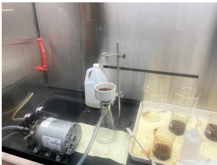
Fig. 5.2: Vacuum filtration using Buchner Funnel inside the fume hood.
