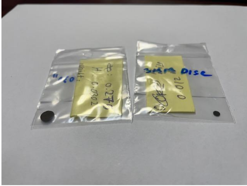
Fig. 5.18: Fabricated disk after pressing with a 2.5-ton hydraulic press machine.
