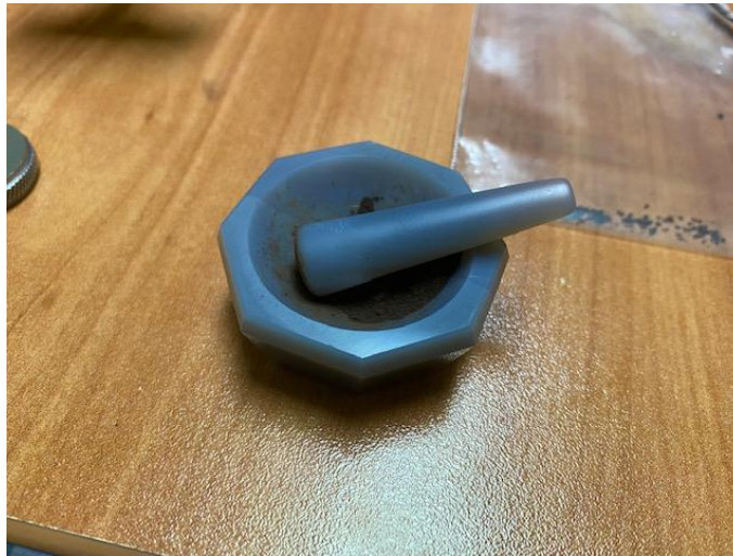
Fig. 5.15: Fabricated ferrite powder after grinding with mortar & pestle.
