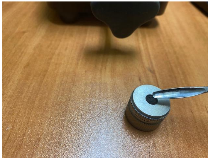
Fig. 5.16: Fabricated ferrite powder inside die-set with isopropyl alcohol.
