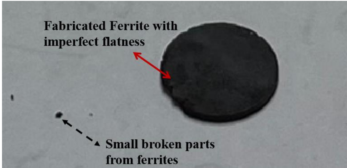
Fig. 5.39: Fabricated non-flat ferrite disk.
