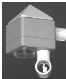
Figure 2: 260-700-D Ultrasonic Snow Depth Sensor [39]
