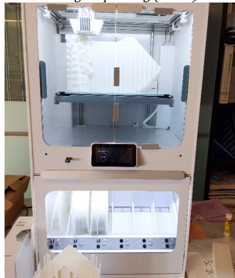
Figure 4.2.7: The Ultimaker S5 3D printer nearing completion on the printing the part
