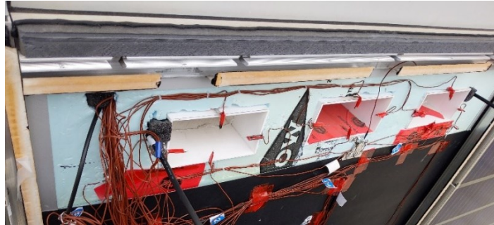
Figure 3.1.5: Thermocouples placed symmetrically around the manifold inlet opening to measure average manifold inlet air temperature.
