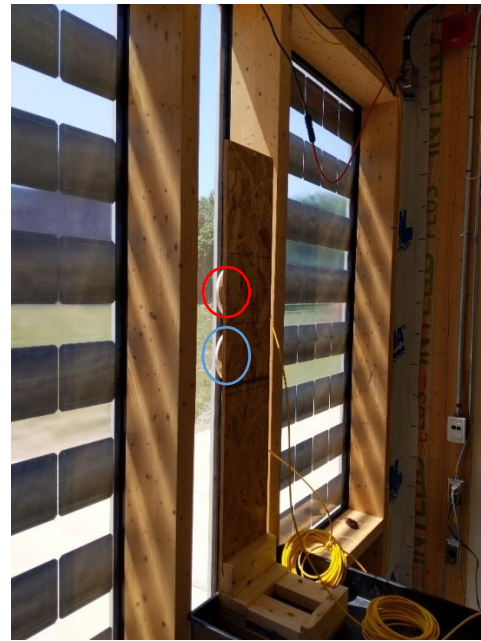
Figure 6.2.7: Indoor SMP22 Pyranometer (in red) and SGR4 Pyrgeometer (in blue) mounted on a wooden stand.
