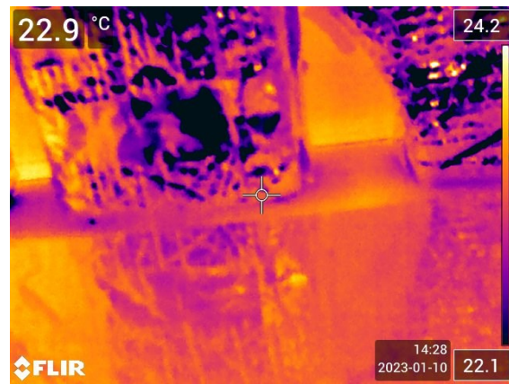
Figure 4.2.16: Infrared imaging of BIPV/T manifold showing more minor thermal bridging effects near the perimeter of the middle manifold inlet
