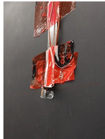
Figure 3.1.4: One thermocouple fixed to black aluminum using foil tape to measure the back pan
