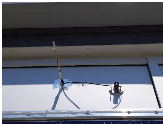
Figure 3.1.9: Type T thermocouple fixed to a wooden stick on the left, LI-COR LI-200 pyranometer on the right.
