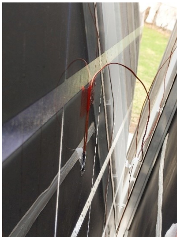
Figure 3.1.3: Thermocouple fixed to the back of the PV module, positioned at the center of the PV cell
