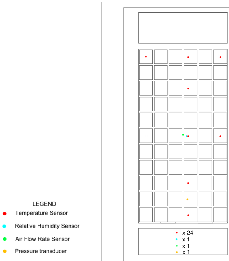
Figure 3.1.7: Positions of monitoring sensors in elevation view
