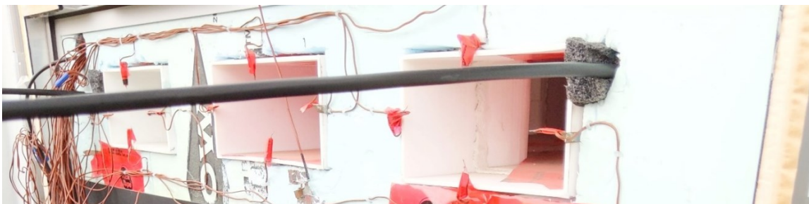
Figure 4.2.19: Four Type-T thermocouples at each manifold inlet to measure temperature of the air stream
