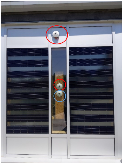
Figure 6.2.6: SMP22 Pyranometers (in red), one on the exterior, one interior, and SGR4 Pyrgeometer (in blue).
