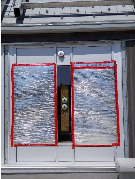
Figure 6.2.11: Reflective insulation applied to the exterior of glazing units not being tested.
