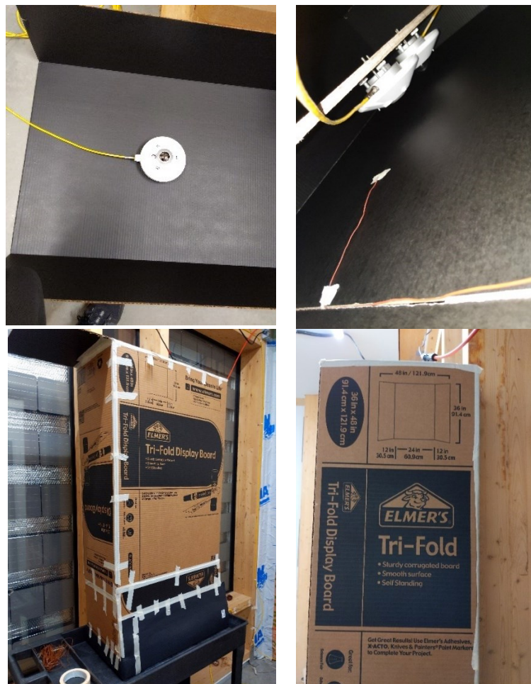
Figure 9.17.1: SGR4 test setup inside the black Tri-Fold cardboard box enclosure
