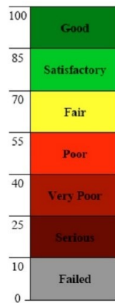
Figure 1-2 Standard PCI rating scales and suggested colors for their representation [6]
