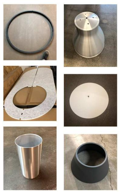
The components were mostly made of aluminum, some from steel. They each had their own finishes: clear coats, powder coating or anodization. Some had pre-cut holes or built in bolts in preparation for assembly. The components shared characteristics of
