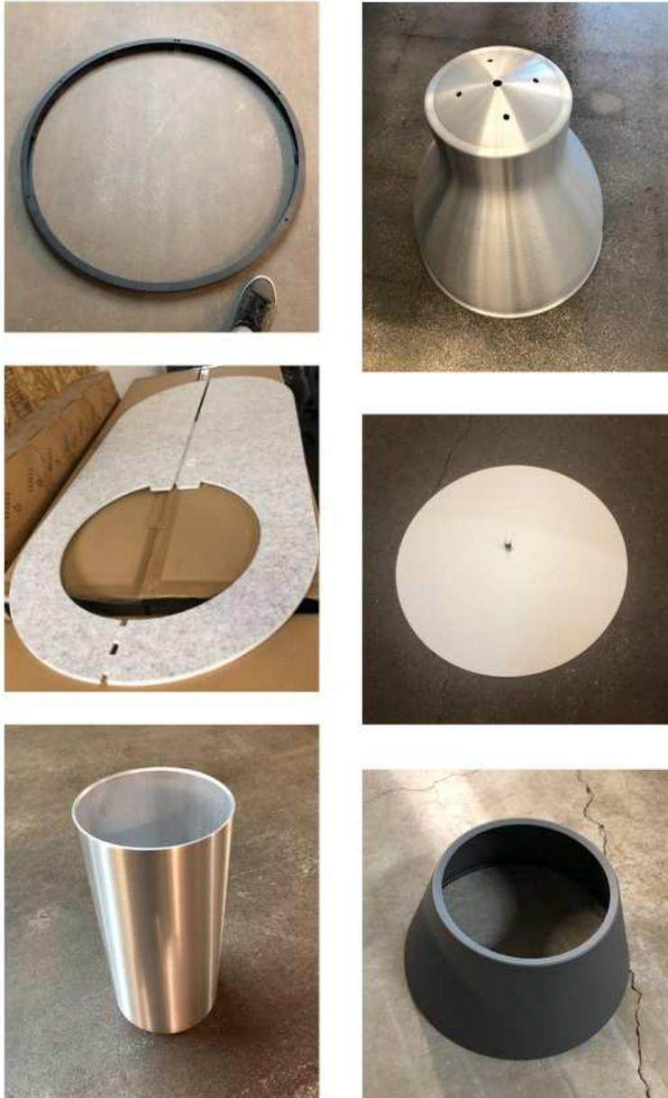
The components were mostly made of aluminum, some from steel. They each had their own finishes: clear coats, powder coating or anodization. Some had pre-cut holes or built in bolts in preparation for assembly. The components shared characteristics of
