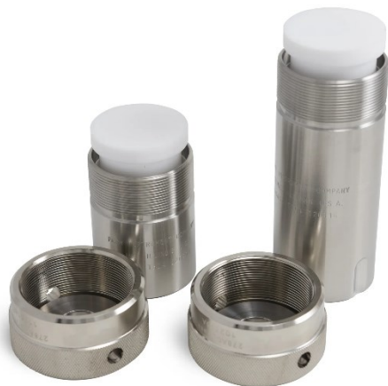
Figure 17. Teflon-lined stainless-steel bomb hydrothermal reactor
