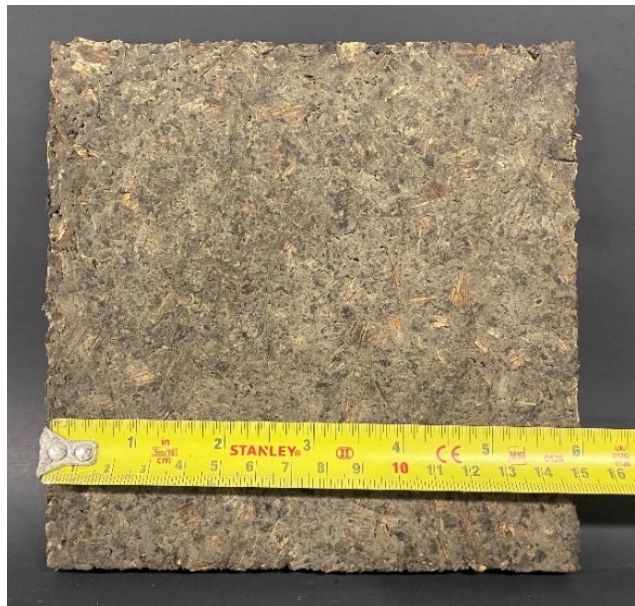
Figure C. 4 The final product quality and dimension after 24hrs. of steam curing
