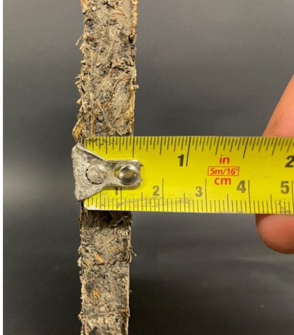
Figure C. 5 The product's thickness after 24hrs. of steam curing
