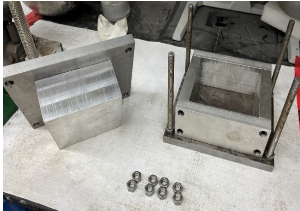
Figure C. 3 The designed mold for producing cement-bonded particleboard.
