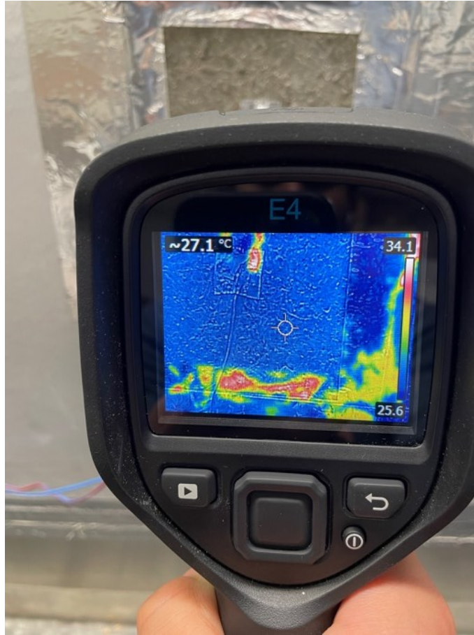
Figure C. 20 Thermal photo of the CBPB captured with FLIR camera
