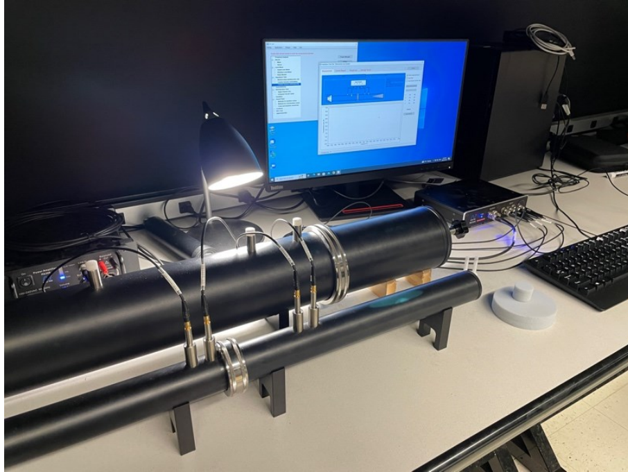
Figure C. 6 Sound insulation test setup
