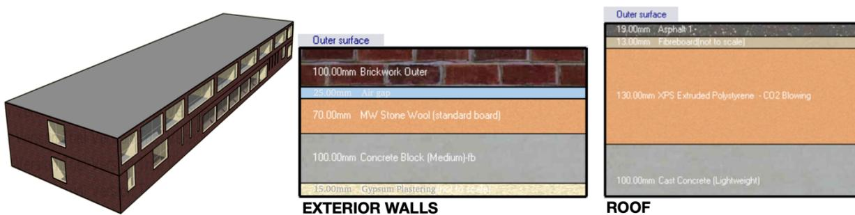
Figure 16. Pre-retrofit design, exterior walls, and roof layers.
