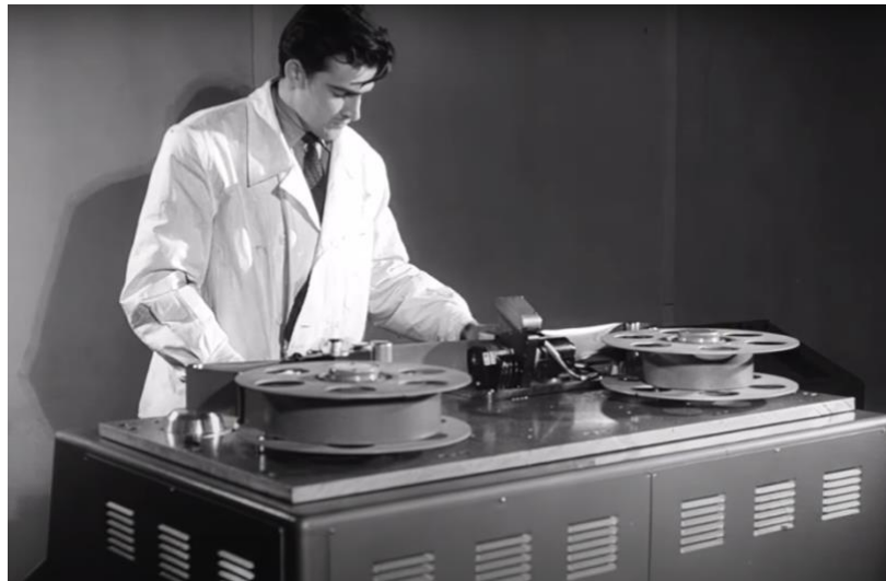
Figure 1.3. The First Soviet ‘VCR’, KMZI-1. Screen grab from the documentary Videomagnitofon (1963), uploaded by Vidachestvo Archive , accessed August 1, 2023, https://www.youtube.com/watch?v=B-WxAGTp6Ig .
