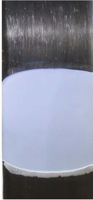
b. Under flow with slip (time=4.8 s)
