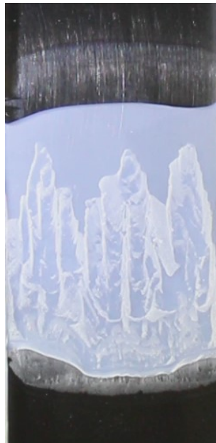
f. Rupture propagation (time=14.2 s)
