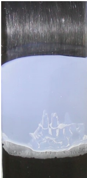
e. Rupture propagation and merging the finger-like streamlines (time=7.6 s)
