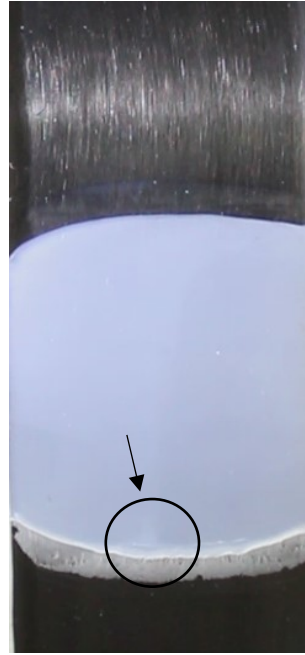
c. the onset of rupture with a finger-like streamline (time=5.9 s)
