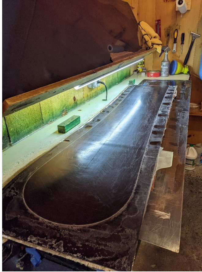
Figure 3.10 - Unfinished snowboard before grinding [39]
