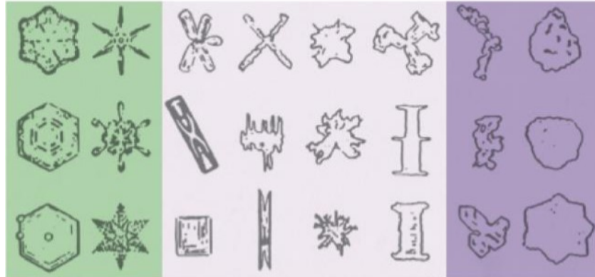
Figure 3.8 - Snow grain shapes from most abrasive (left) to least (right) [32]
