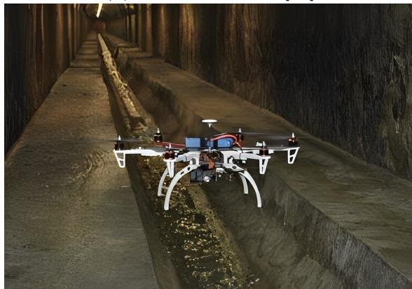
(f) Sewer Inspection [35]
