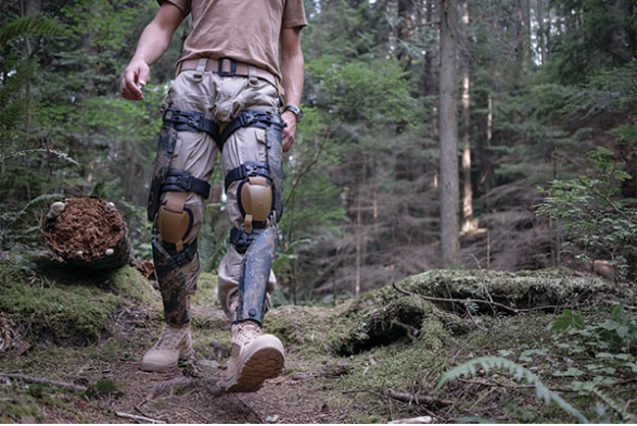
(c) Strap-on kinetic energy harvester from walking [15]
