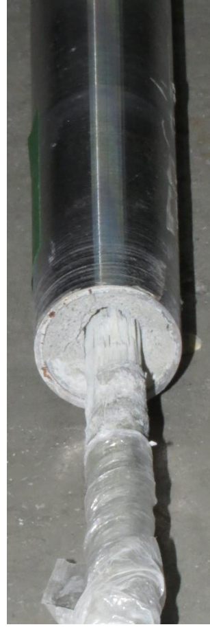
(c) Longitudinal cracks beside the grip
