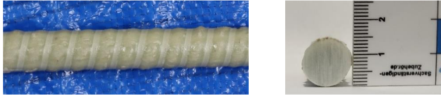
Fig. 4.2. Ribbed GFRP bar
