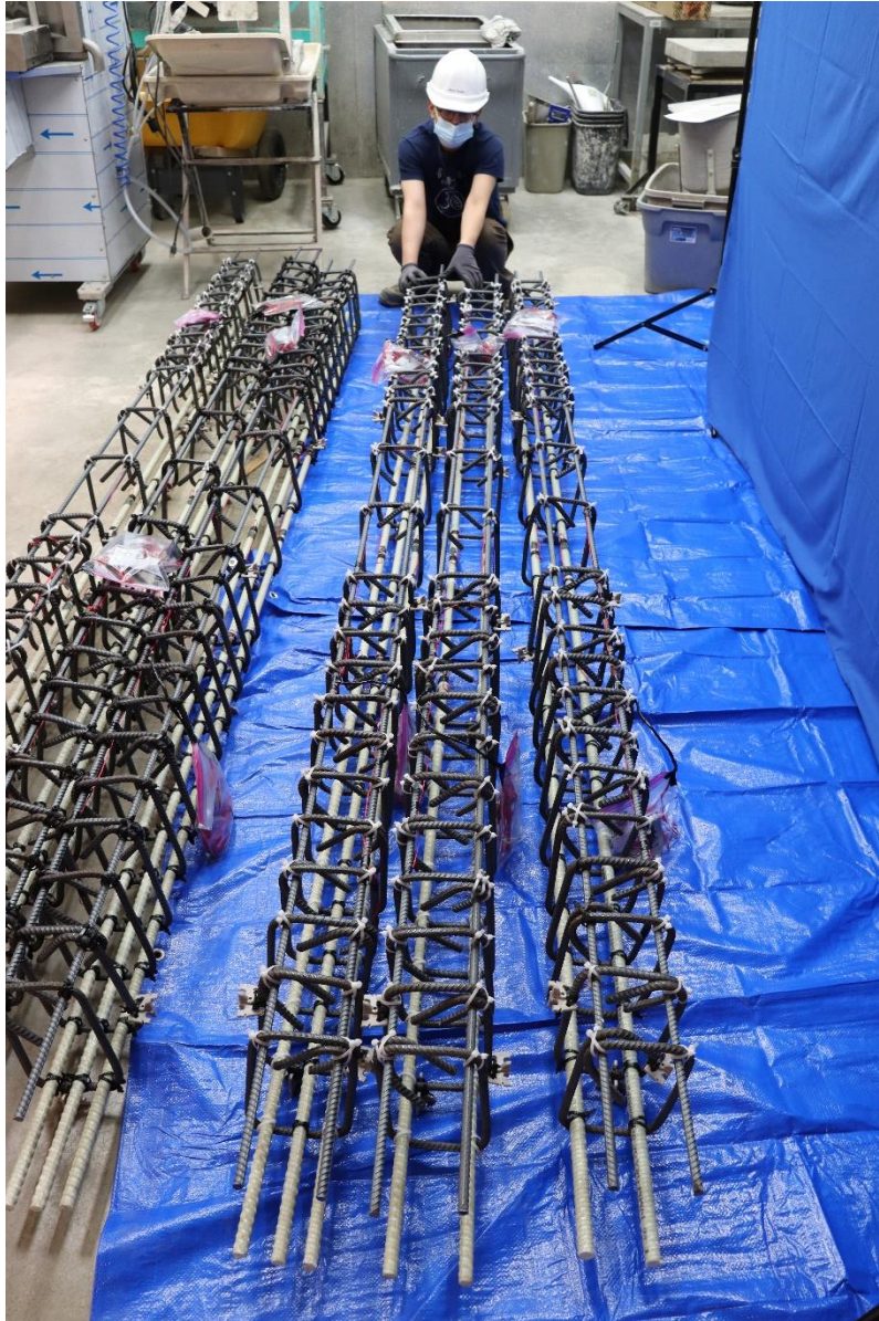
Fig. A.1 Typical GFRP cages for concrete beams
