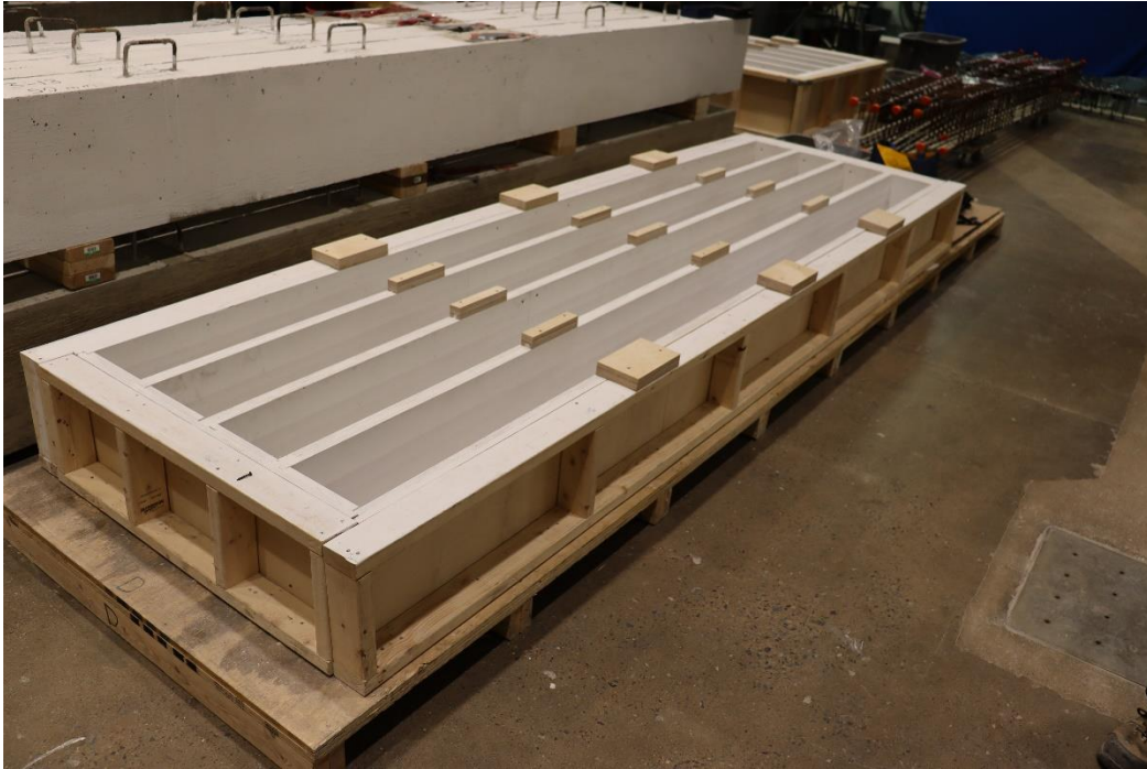
Fig. A.2 Typical formwork for the concrete beams
