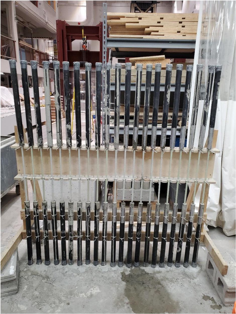
Fig. A.6 Pouring grout to grip the GFRP bars.
