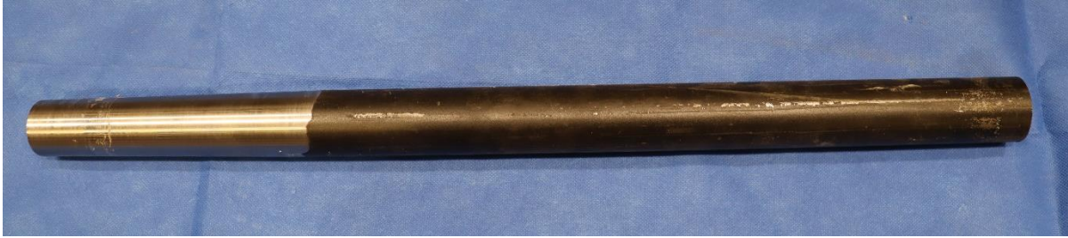
Fig. 4.5. Steel tubes used for fatigue testing
