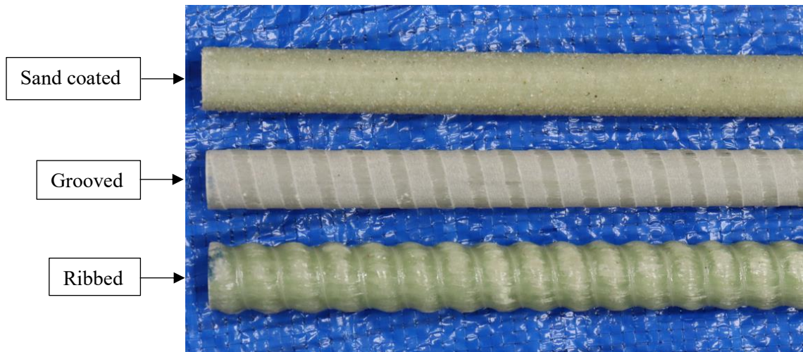
Fig. 1.1. Common types of GFRP bar surfaces
