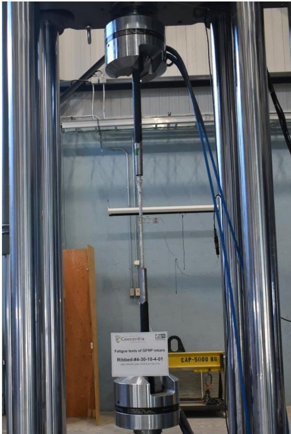
(a) Not failed GFRP bar after fatigue loading
