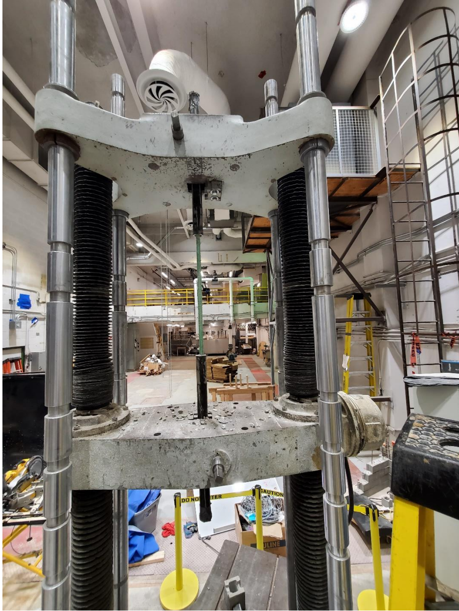
Fig. A.7 Testing GFRP bar under low cycle fatigue
