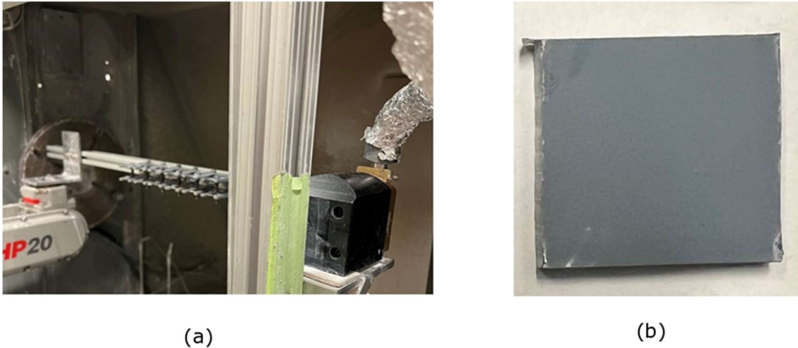
Figure 2-4. The redesigned experimental setup to generate coatings with full cover of substrate. (a) redesigned setup (b) coating covering the substrate completely .
