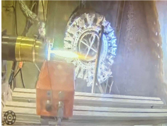
Figure 2-7. Measuring the velocity of in-flight particles with Accuraspray 4.0.
