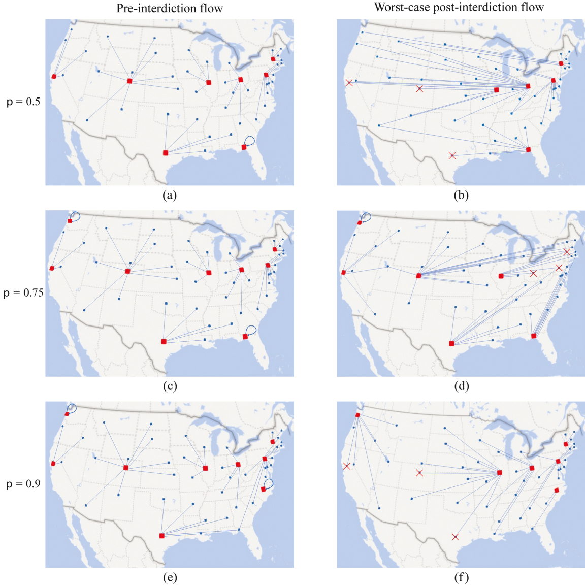
Figure 2.8: Effects of Varying p on the Design for Set I, \rho_2 = 0.5 and B = 3 . (a) Pre-interdiction Flow for p = 0.5 , (b) Worst-case Post-interdiction Flow for p = 0.5 , (c) Pre-interdiction Flow for p = 0.75 , (d) Worst-case Post-interdiction Flow for p = 0.75 , (e) Pre-interdiction Flow for p = 0.9 , (f) Worst-case Post-interdiction Flow for p = 0.9
