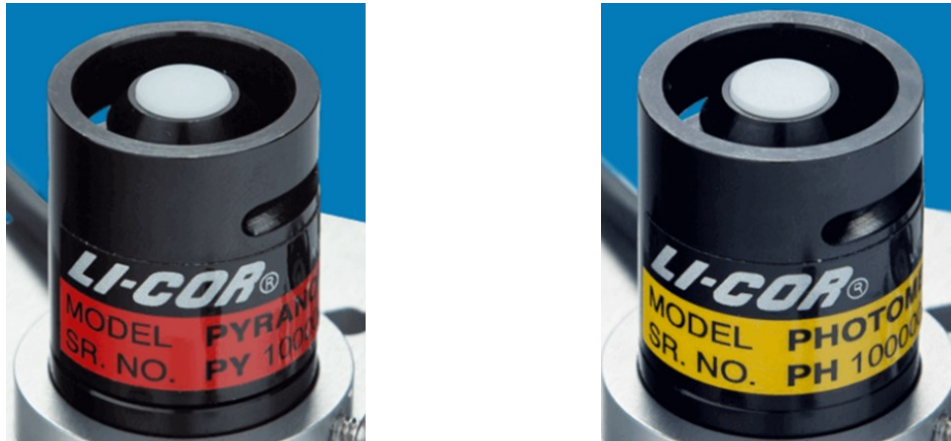
Figure 3.4: Images of the pyranometer and photometer used in the experimental setup (LI-COR, Inc., 2022a; LI-COR, Inc., 2022b).
