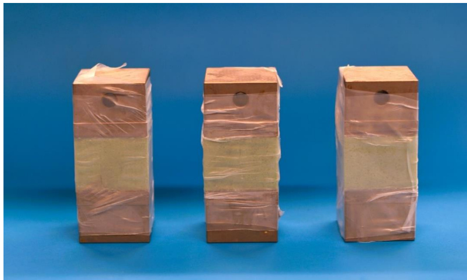
Figure 3.7. Wet samples wrapped with Parafilm M Lab film during the adhesive curing process.
