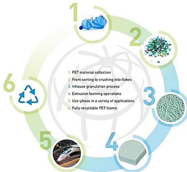
Figure 2.4. Stages of the ArmaPET Struct recycling process [58].
