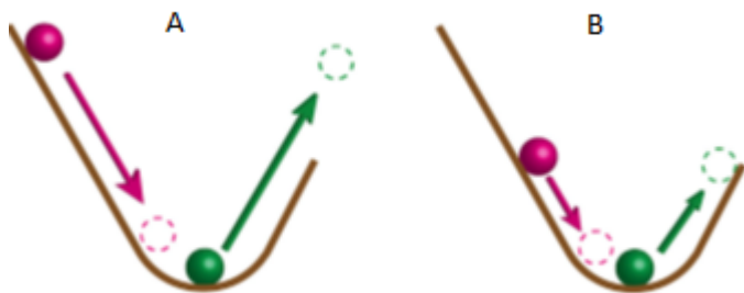
Figure 3: Similarity between gravitational potential energy and redox potential on charge carriers (a) fall from a higher altitude (b) fall from a lower altitude. Reproduced with permission from ref. [35]
