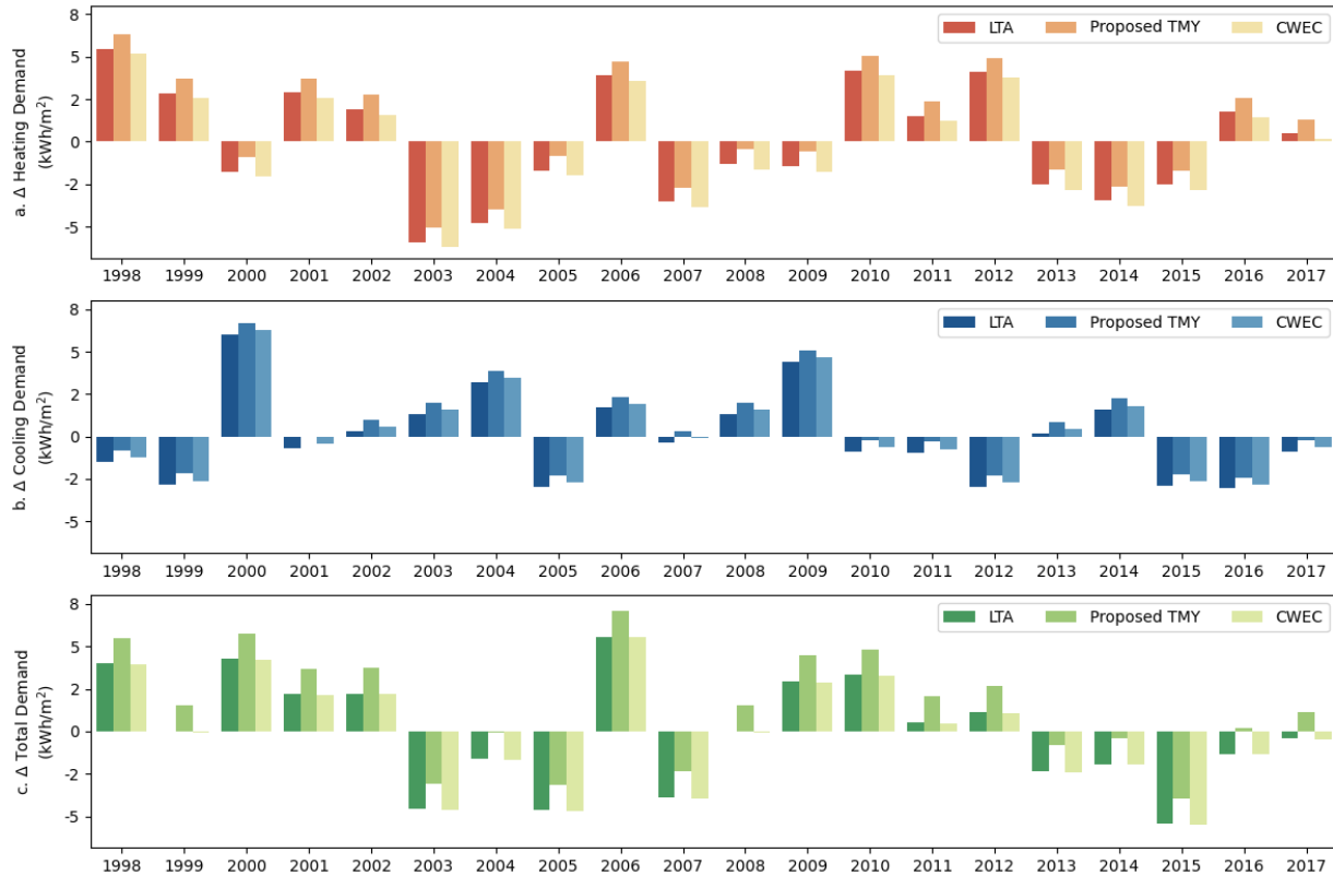
Figure 2.7: Comparison of annual energy demand results for reference year weather files and CWEEDS dataset.
