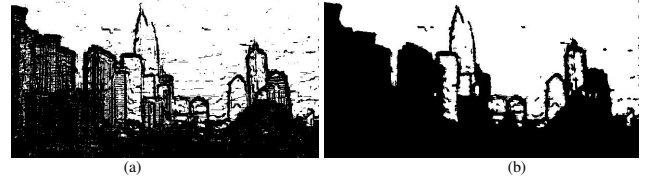
Fig. 3 (a) Binary image in which the black pixels have higher G_M values than white ones. (b) Binary mask generated by the stage of segmentation.
