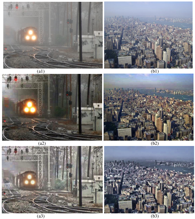
Fig. 7 (a1) (b1) Input images of lightly hazy scenes. (a2) (b2) Haze removed images by DCP [3]. (a3) (b3) Haze removed images by the proposed algorithm.
