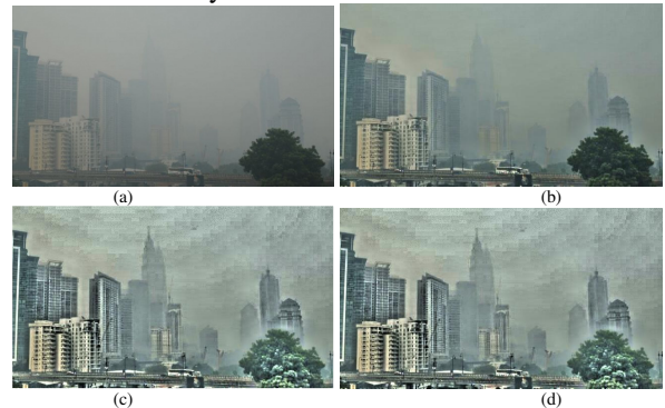
Fig. 1 (a) Example of heavily hazed outdoor image. (b) Result by CLAHE with moderate enhancement. (c) Result by CLAHE with strong enhancement. (d) Result by the method of variable clip limit [2].
