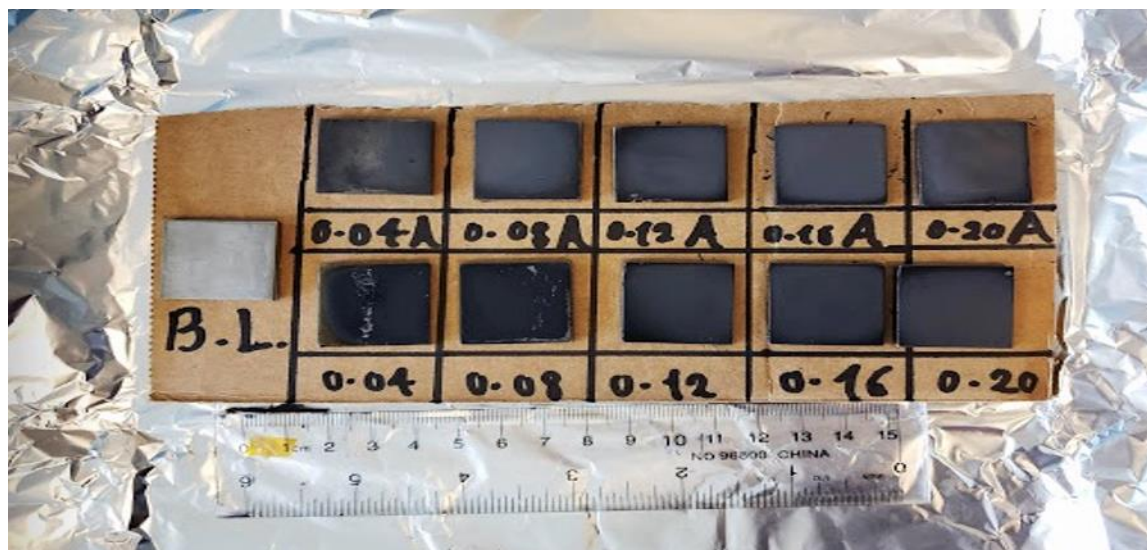
Figure S1. Specimens with photocured coating with the upper row annealed at 190 °C for 2 hours (marked A), and others left untreated. The bare titanium substrate is on the left. The weights of graphene oxide used in the dispersions are shown below each sample.
