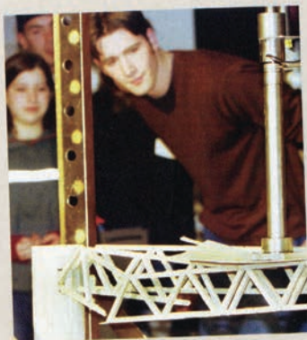
At the 2001 Bridge Building Competition, students watch their bridge sustain "the Crusher," a computer-controlled mechanism with a 10-ton capacity.
