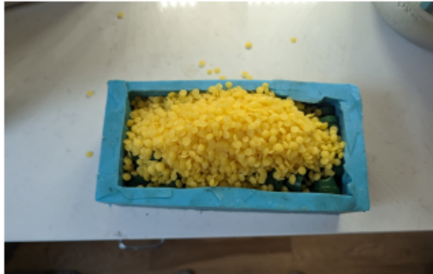
FIG. 32 MOLD FILLED WITH BEE'S WAX AND SPRAY PAINT CAPS BEFORE HEAT
