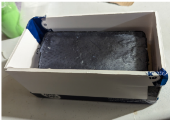
FIG. 29 MOLD CREATED TO RECEIVE SILICON
