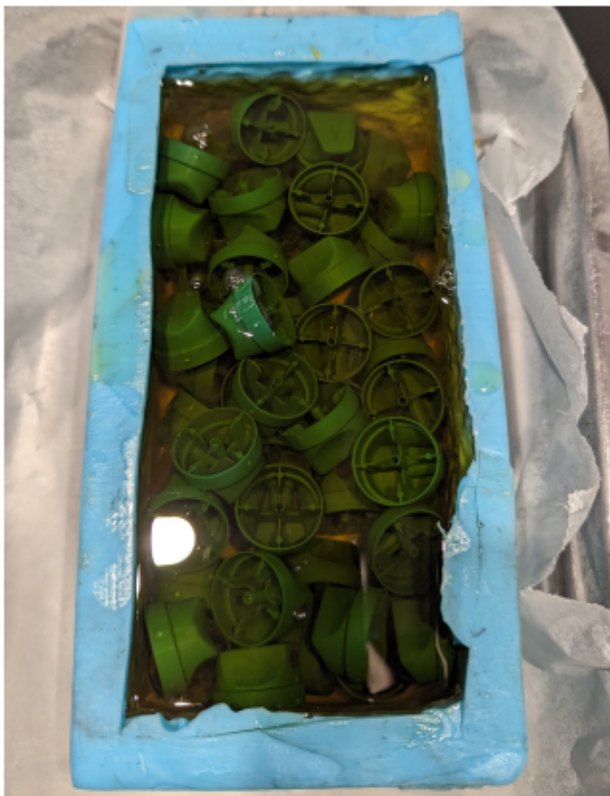
FIG. 33 MOLD FILLED WITH BEE'S WAX AND SPRAY PAINT CAPS
