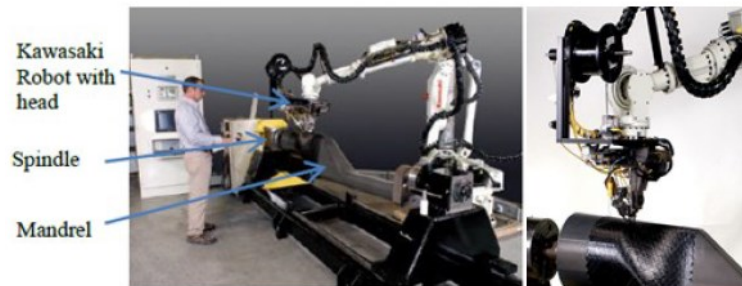
Figure 1.5 A serial manipulator and a mandrel doing a fiber placement [19],[24]
