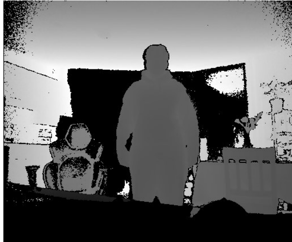
Figure 5 Kinect V2 Depth Image Capture
