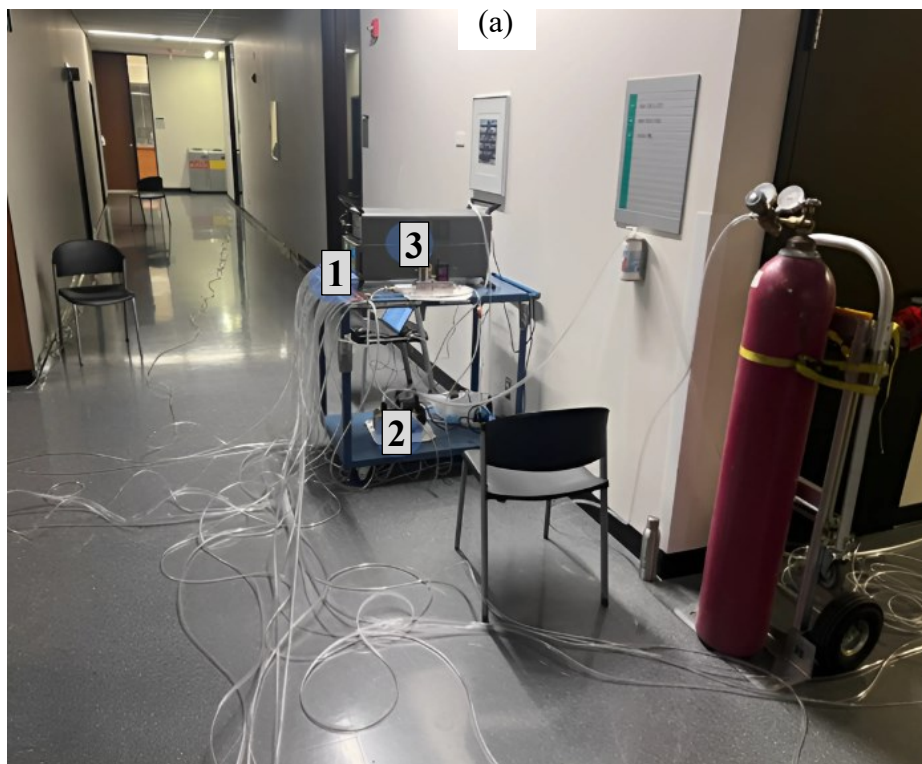
Figure 5. (a) UGA, CO2 cylinder, and sampling tubes in the corridor, (b) Tripods and sampling tubes in room 5670
