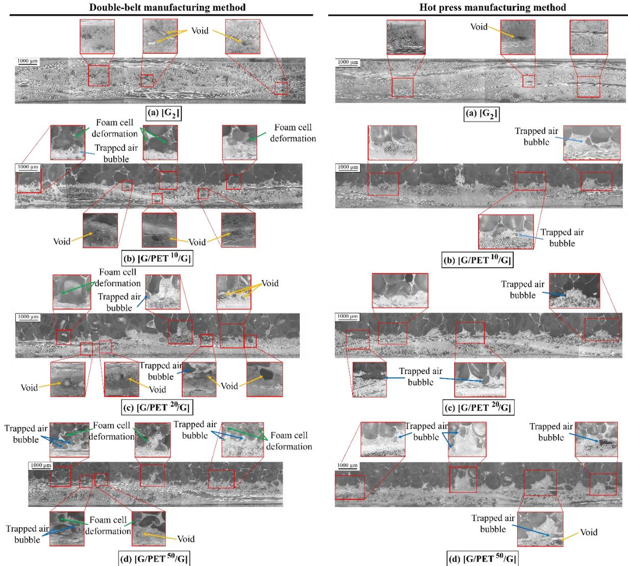
Figure 4.7. Microscopic section views of the (a).  $[G_2]$  composite laminate, and skin-to-core bonding of panels with PET foam thicknesses of (b). 10 mm, (c). 20 mm, and (d). 50 mm.
