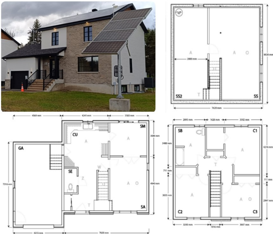
Figure 6.3. Layout of Experimental House for Building Energetics
