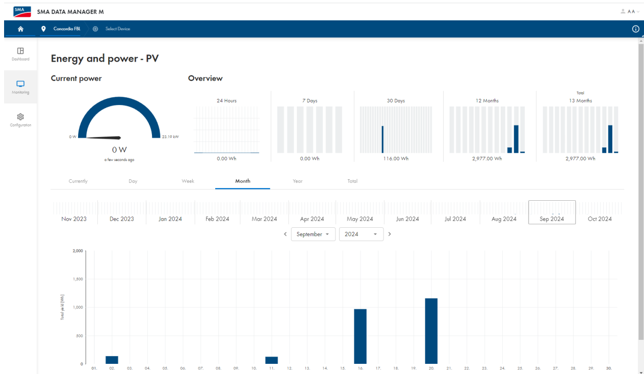
Figure A-10 EDMM PV energy status remote monitoring
