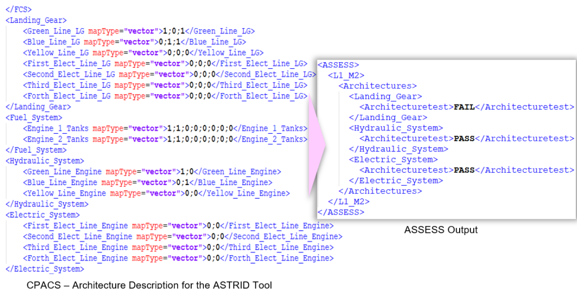
Figure 3.15: Architecture description in ASTRID and corresponding ASSESS output written to the "toolspecific" tag in CPACS
