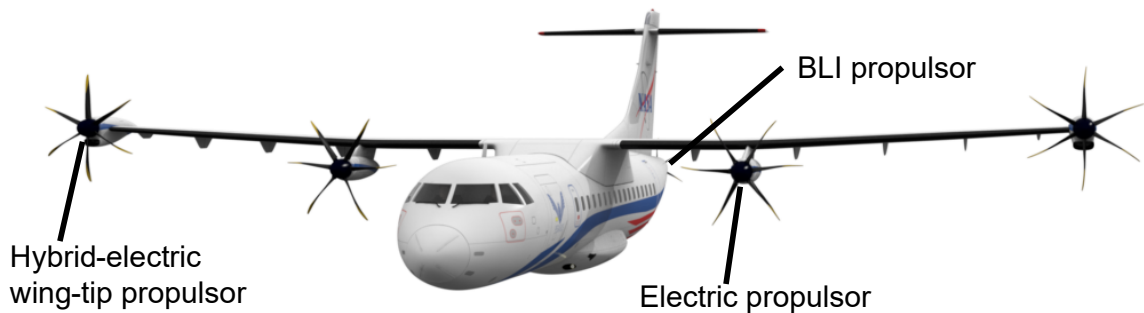
Figure 4.10: NASA Parallel Electric-Gas Architecture with Synergistic Utilization Scheme (PEGASUS) Concept, adapted from [173]
