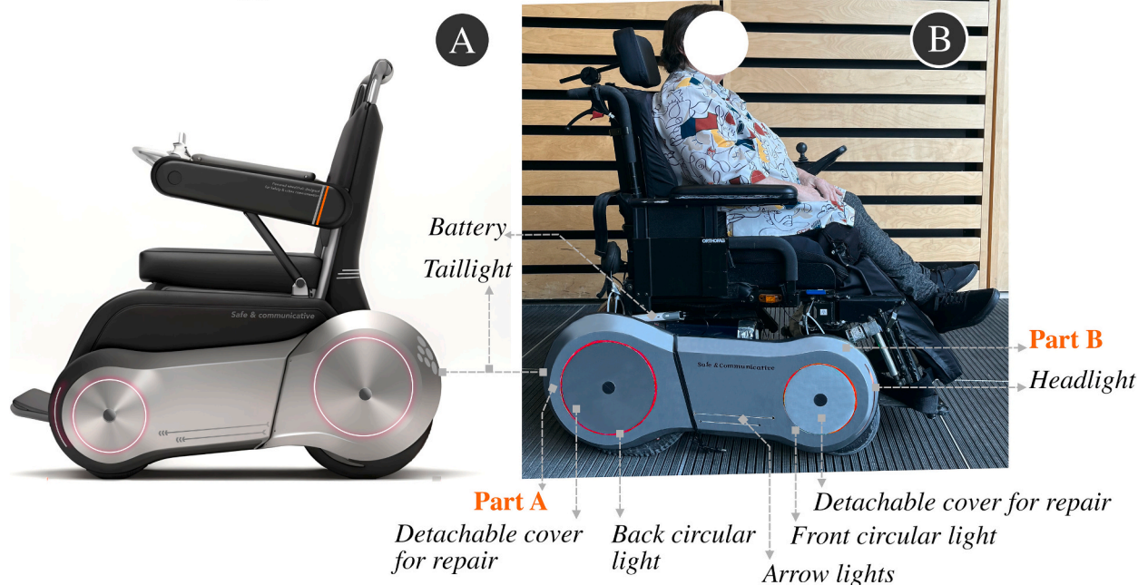
Fig. 6. The final Concept 2: 3D modeling presentation of WheelSafe Illumina. B: Prototype presentation.
