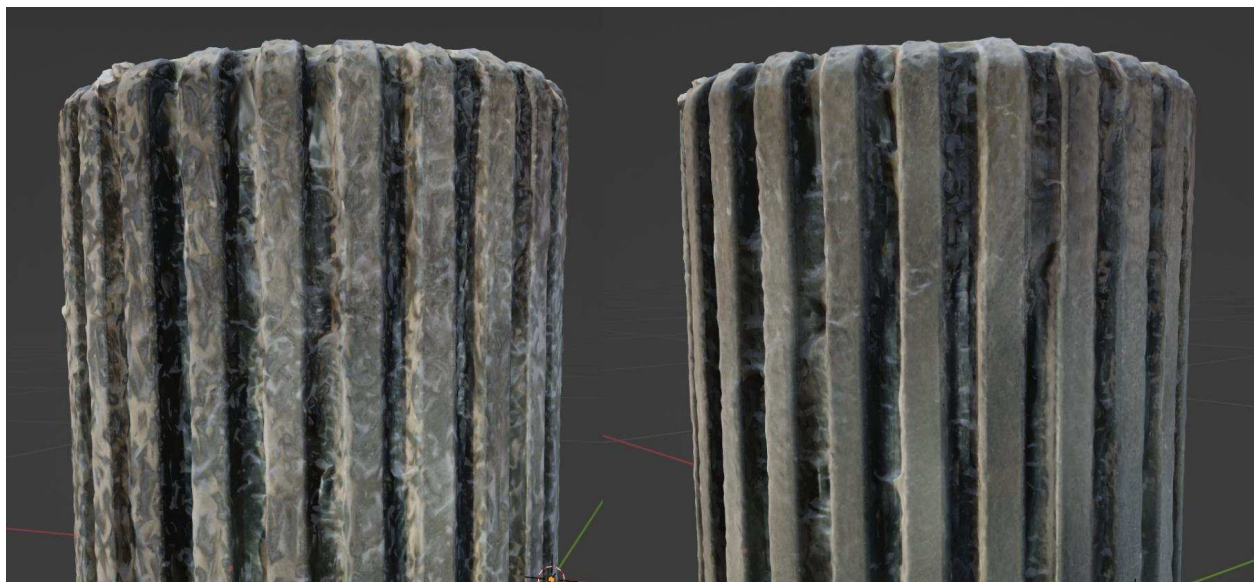
Figure 5.11 - After vertex merging. Custom split normals (left), custom split normals cleared (right).
