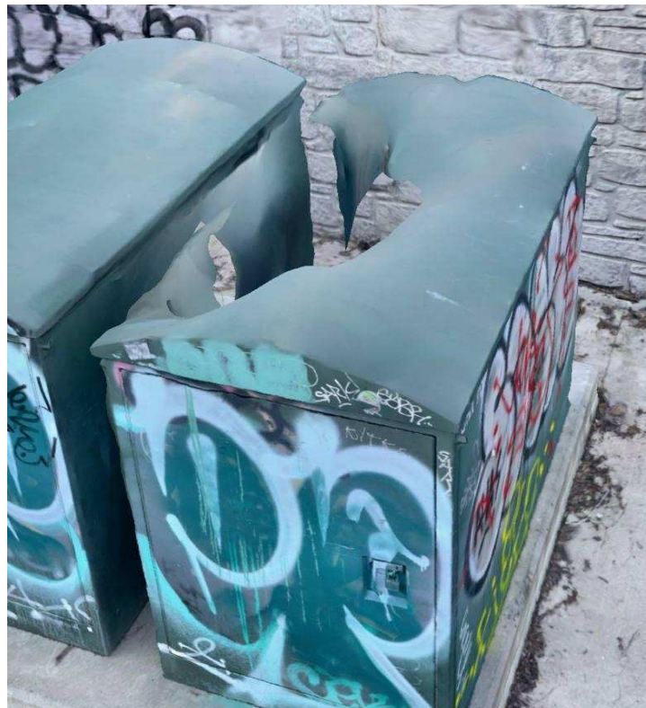
Figure 3.5 - Imperfections of a scan viewed in Polycam.
