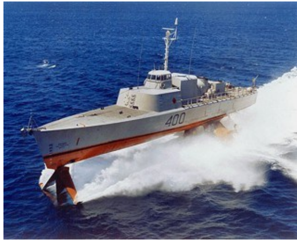
Figure 1.1. HMCS Bras d'Or, a hydrofoil that served in the Canadian Navy in the 1960s [5]
