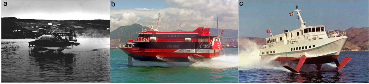
Figure 2.3. a) Bell Hydrodome, b) Boeing Jetfoil, and c) Supramar PT 50 [23]
