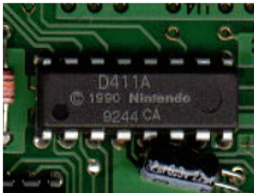
Figure 6.30. An official Nintendo CIC chip, embedded on a PCB.
