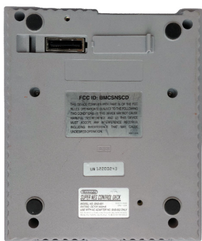
Figure 5.2. The EXT port on a Super NES, with the plastic cover removed.
