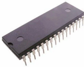
Figure 6.29. An AS6C1008 SRAM chip.
