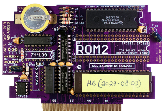
Figure 6.38. The front of my HyperBound reproduction PCB, in its final form.
