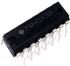
Figure 6.32. A 74HC139 decoder, one of many compatible with the SNES/SFC.
