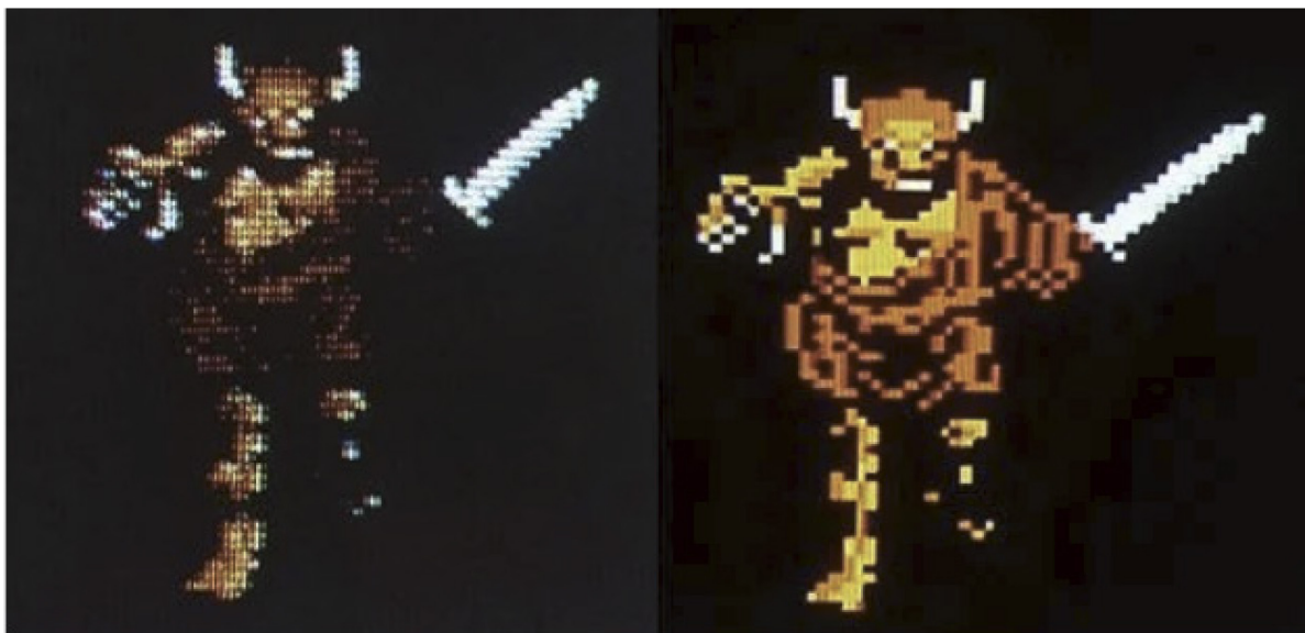
Figure 4.21. A comparison of a NES/FC game sprite, photographed on a CRT and screen captured from an emulator. Photo credit: Benj Edwards.
