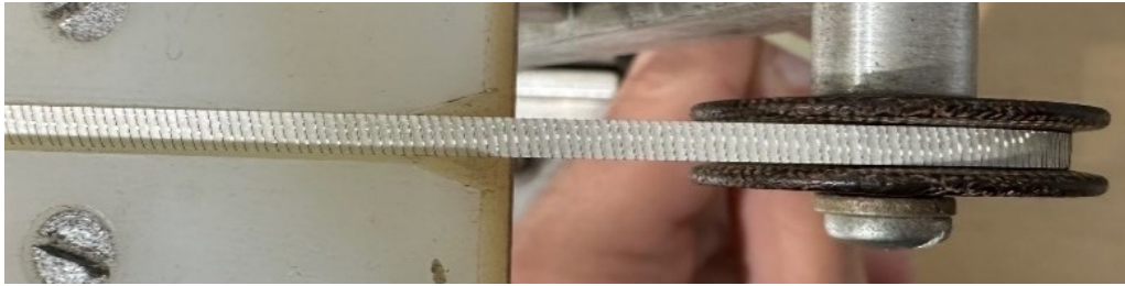
Figure 2.2 shows platinum wires wound around a rectangular paper core
