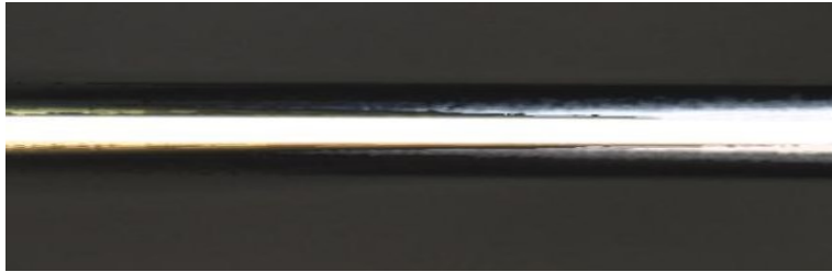
Figure 3.3: Schematic chemically removed coating without any deformation and damage to platinum.
