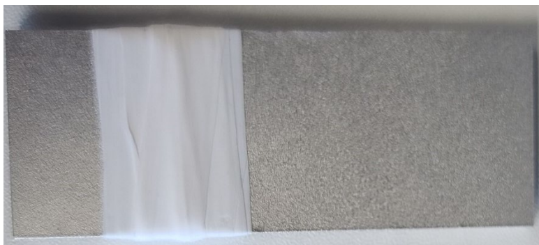
Figure 3. Masking the sample with the Teflon tape.
