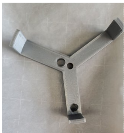
Figure 3. 5custom 3D-printed electrode holder
