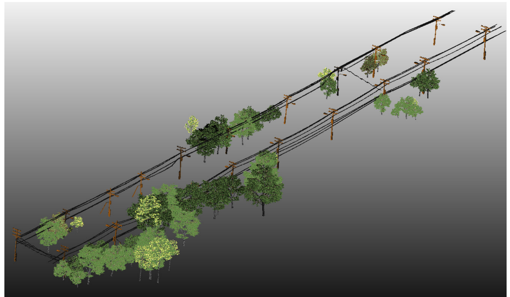
Figure 9. Three-dimensional model of trees, poles and power lines based on point cloud data.
