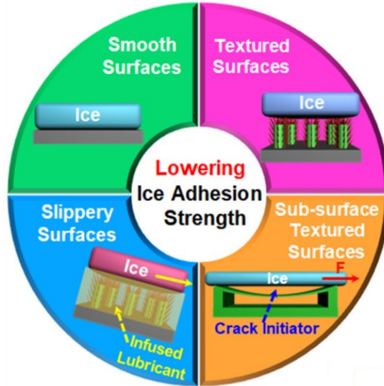
Figure 2.1: Overview of primary strategies for designing icephobic surfaces, categorized by surface properties: smooth, textured (e.g., hierarchical), slippery, and subsurface textured He et al. (2021) .
