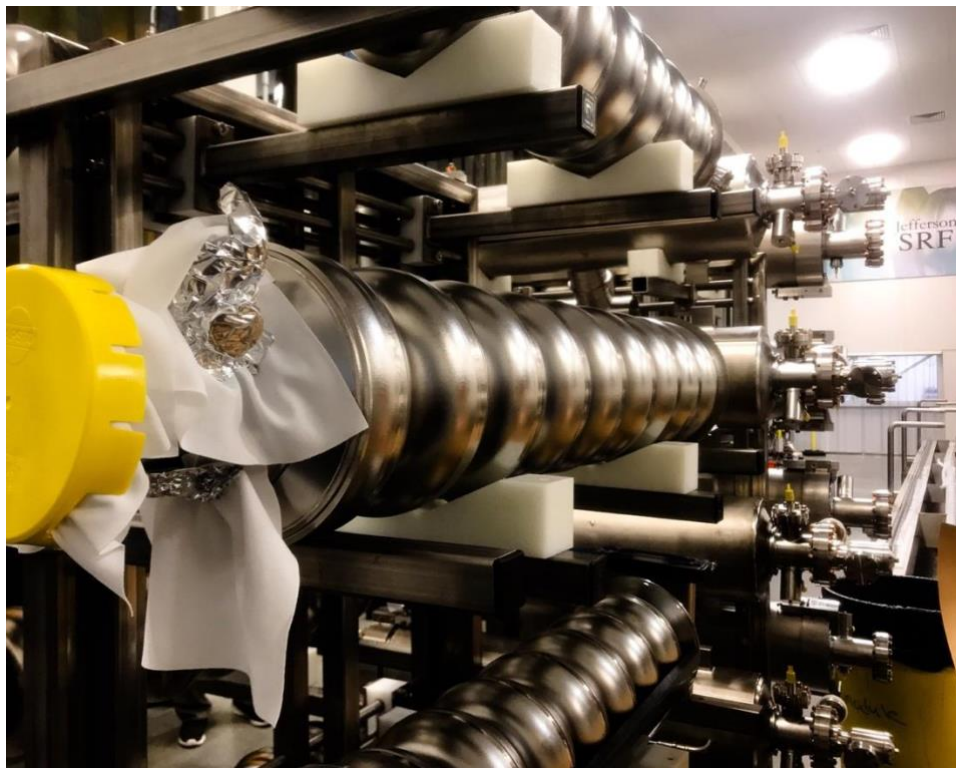
Image 4.1 Niobium bulk SRF cavities produced at Jefferson Lab, in Virginia, USA. (Salas, A., 2024).
