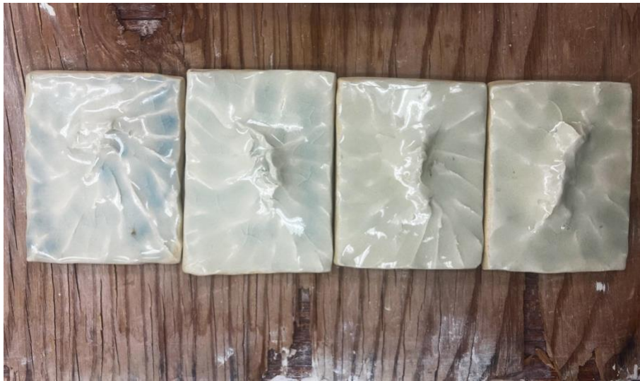
Image 5.5 Test tiles with niobium-based glaze at Banff. (Salas, A., 2024).
