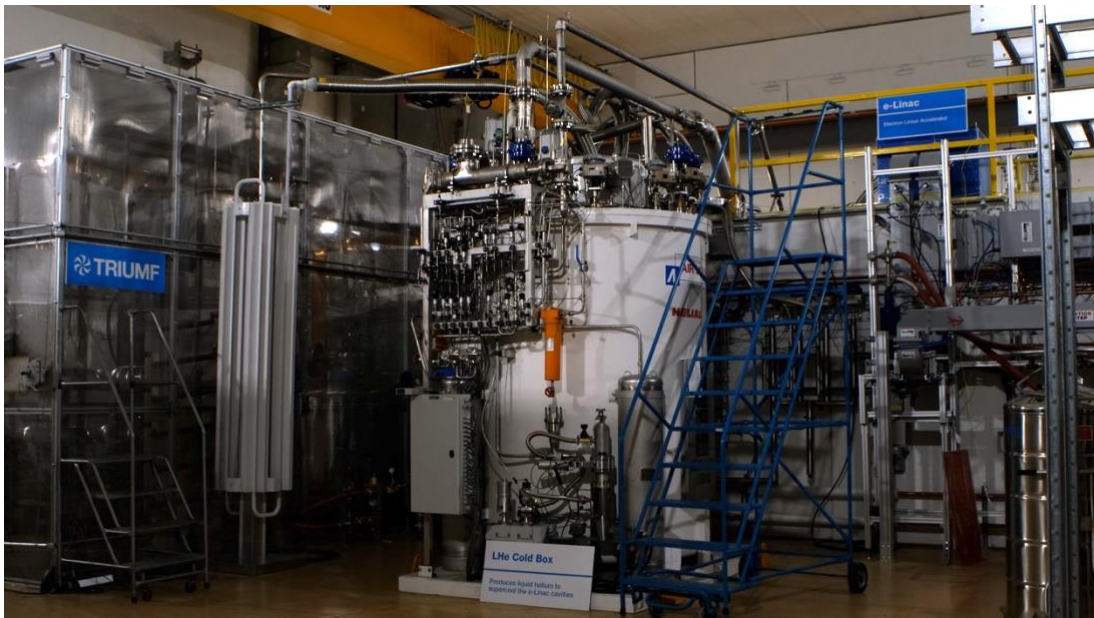
Image 3.5 Linear Accelerator Cold Box at TRIUMF. (Salas, A., 2024).
