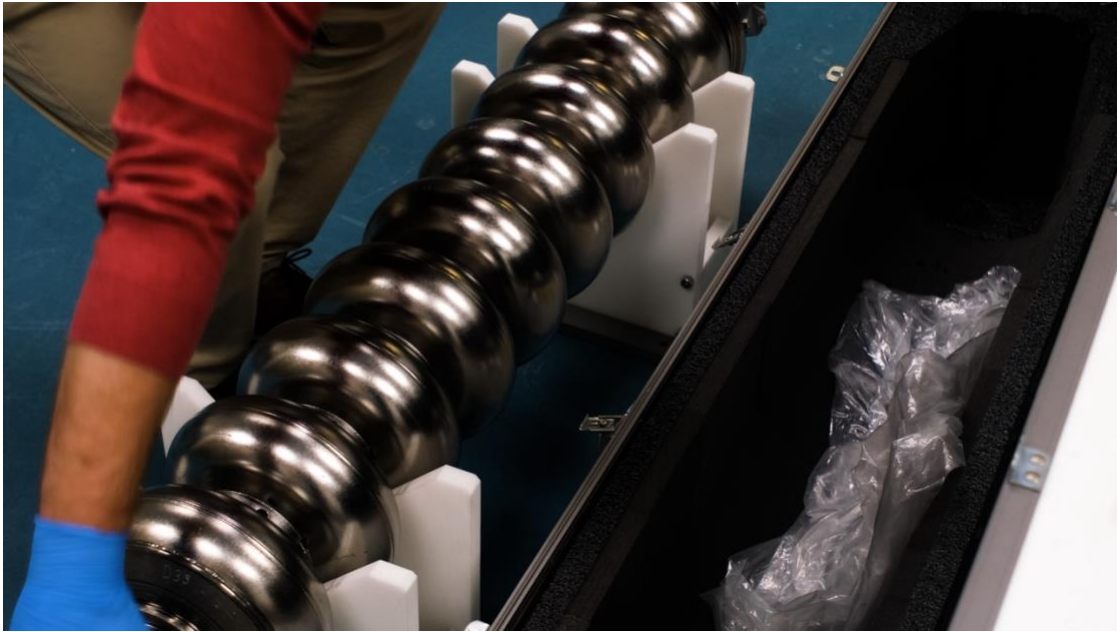
Image 5.2 SRF Niobium Cavity at TRIUMF. (Salas, A., 2024).
