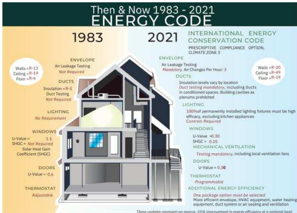
Figure 3.2 Changes in building energy code standards in Canada (1983–2021). Source: Energy Codes Then and Now: 1983–2021 , Sustainable Energy Action. Last accessed January 16, 2026 from https://sustainableenergyaction.org/resources/energy-codes-then-and-now-1983-2021
