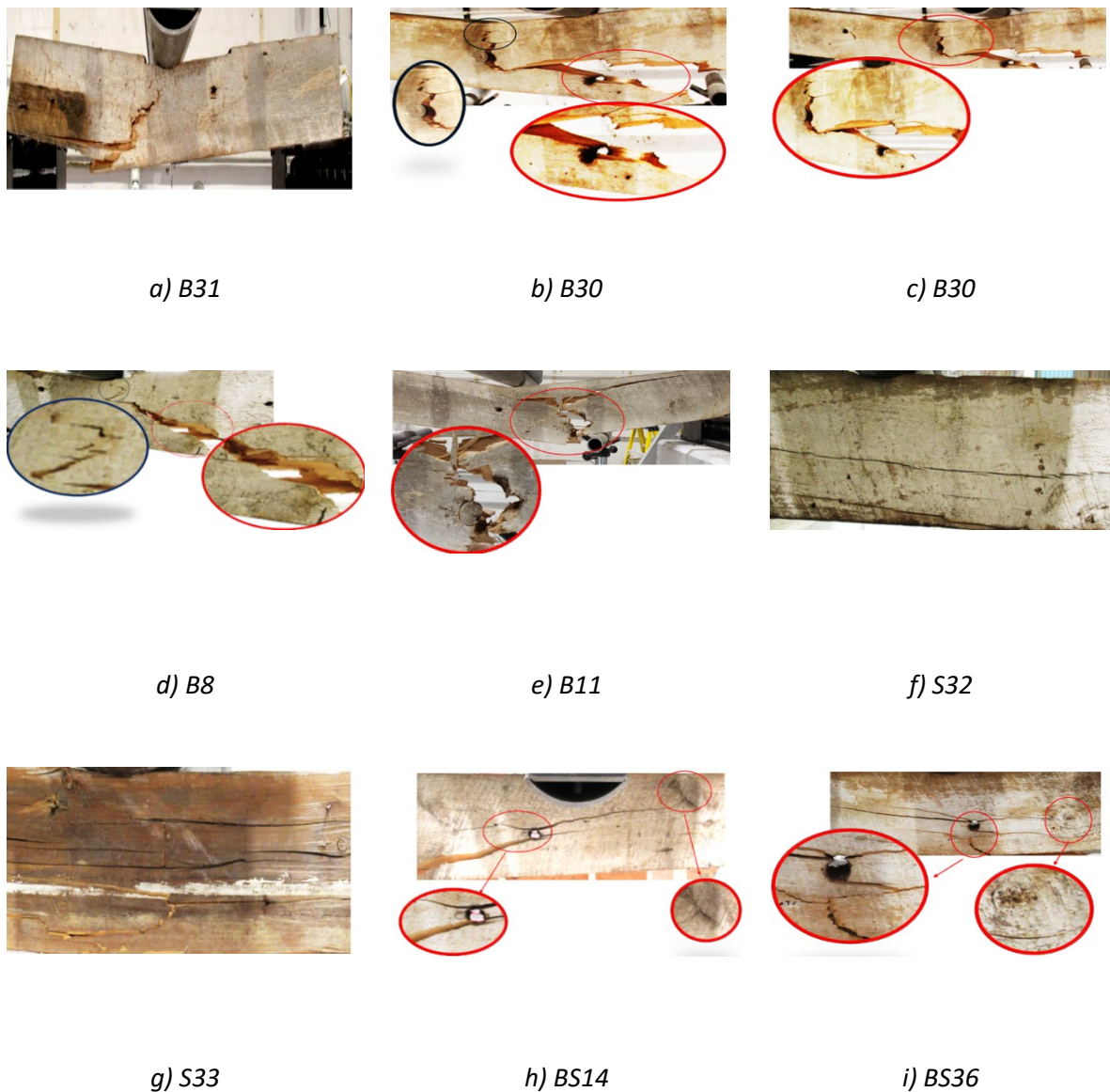
Fig. 3.7. Visual shear, flexural, and coupled failures
