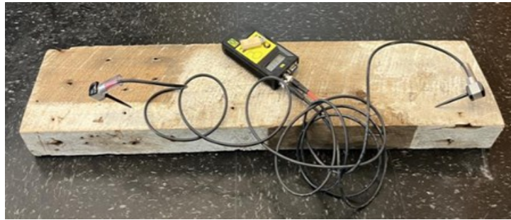
Fig. 3.1. Non-destructive tests (Ultrasonic measurements)
