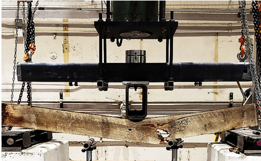
Fig. 3.2. Destructive tests on Heritage beams
