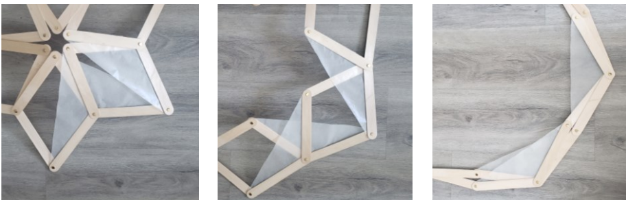
Figure 29. Expansion sequence— Attaching rigid plates to the two pantographs of prototype 5 (Hor, 2024).
