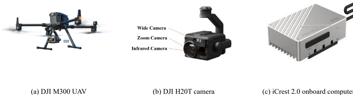
Figure 1-2 Early wildfire detection and suppression hardware system
